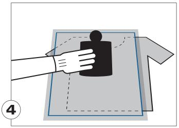
Cover the Phadebas® paper with a clean glass board. Weigh down the arrangement.
