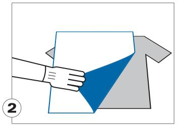
Cover testing area with Phadebas® paper, reagent side down. Dampen Phadebas® paper with water.
